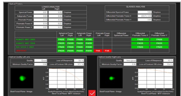
Optical Quality Check (Option): Measurement the quality of the lens (Loss of Sharpness and Contrast)
