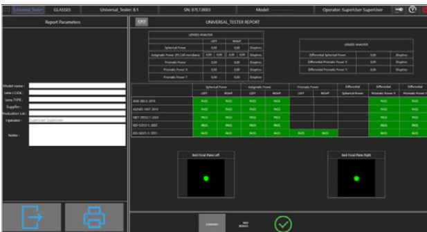
Refractive Power Check: immediate display of the test result with the power values
