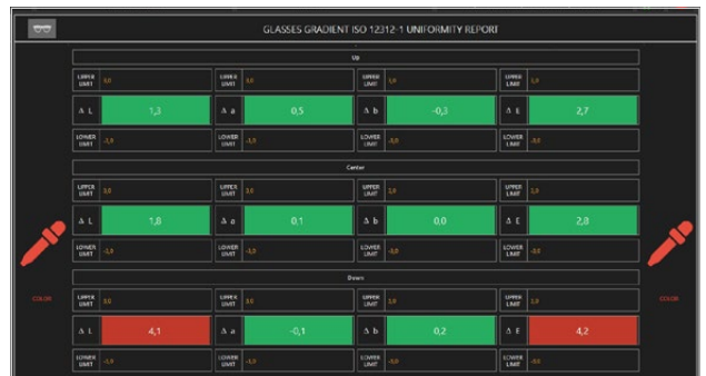
Color Matching Option: System check the colorimetric differences in terms of estimated \Delta L , \Delta a , \Delta b and \Delta E
