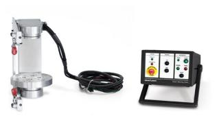
Smart\_Rotating\_Robot with the control unit allow quality control of cylindrical components and any other item that needs to be examined on different projection planes at defined angles.
