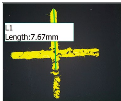
Dimensional check on a surface
