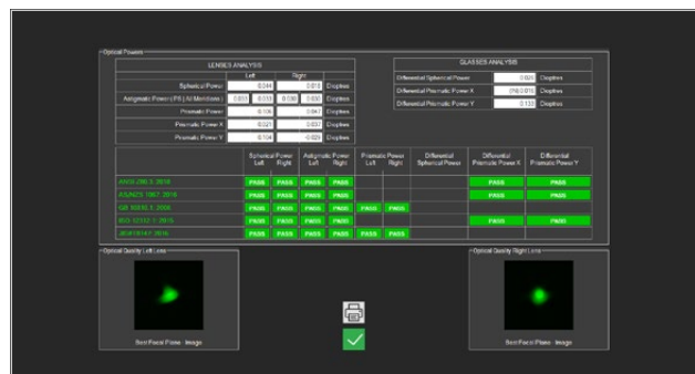
SunGlasses & SkiGoggles: configuration with a Smart_HeadForm tool to measure Optical Quality and Refractive Powers for SunGlasses and SkiGoggles. The stage is movable to measure the both left and the right lens.
