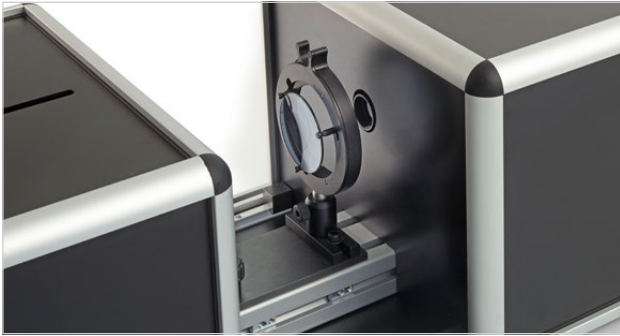
SunLenses: configuration to measure Optical Quality and Refractive Powers for SunLenses. Lens_Holder tool allow self-centering position of lenses with diameters up to 80 mm.
