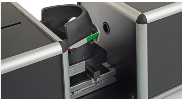
SunGlasses & SkiGoggles: configuration with a Smart_HeadForm tool to measure Optical Quality and Refractive Powers for SunGlasses and SkiGoggles. The stage is movable to measure the both left and the right lens.
