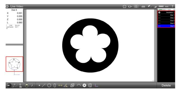
Thanks to the **Smart\_Wire\_Measurement** insulation tool it is possible to determine the number of strands in a wire automatically, as well as manually select the appropriate figure.
