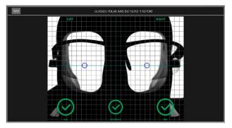
**Polar Axis Check:** immediate display of « Pass / Fail » test result, including report with all data
