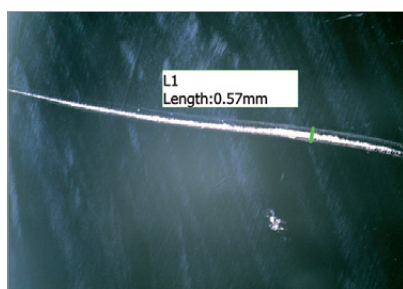
Scratch measurement on glass
