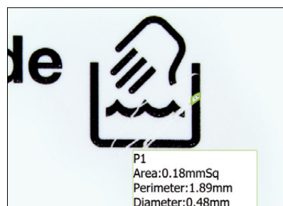
Scratch measurement on a surface
