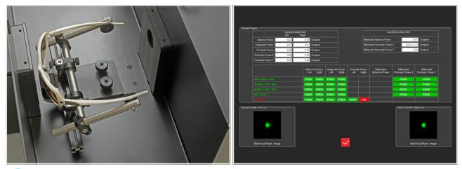
**Smart\_OptiBench XXL SunGlasses**: configuration with flexible fixing tool to measure the Optical Refractive Properties and the Optical Quality of SunGlasses with frame. Free interaxle spacing between SunGlass Lenses.
