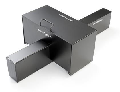
"Smart\_OptiBench XXL automatically checks the Optical Powers of SunLenses, SunGlasses with frame, Masks and Visors"
